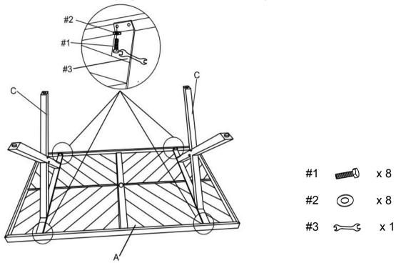
Step 2. Attach table connector (part B) to table legs (part C) using bolts (part #1), flat washers (part #2) and wrench (part #3).
