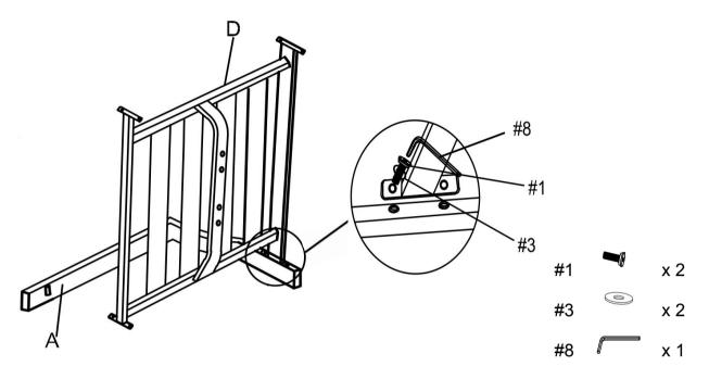
Step 2. Attach left arm (part B) to seat panel (part D) using bolts (part #1), flat washers (part #3) and allen wrench (part #8).
