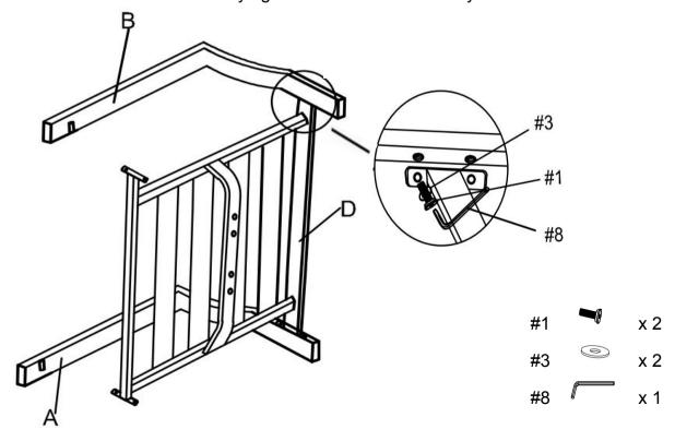
Step 3. Attach back panel (part C) to assembled unit (parts A, B & D) using bolts (part #1), long bolts (part #2), flat washers (part #3) and allen wrench (part #8).
