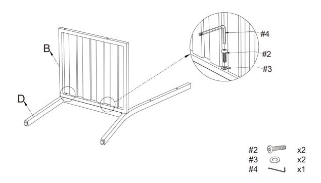
Step 2. Attach back panel (part A) to left arm panel (part D) using bolts (part #1), flat washers (part #3) and allen wrench (part #4).
