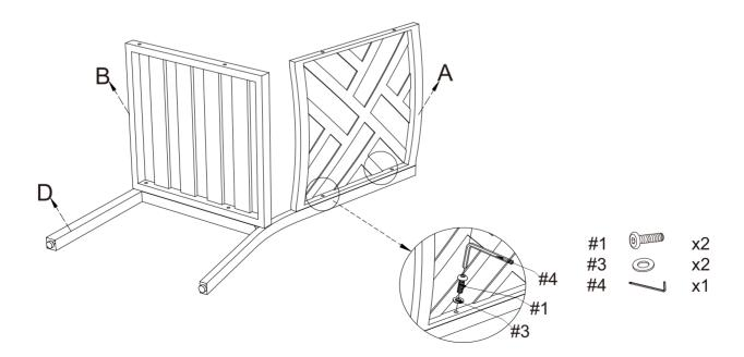
Step 3. Attach right arm panel (part C) to back panel (part A) and seat panel (part B) using bolts (part #1), long bolts (part #2), flat washers (part #3) and allen wrench (part #4).
