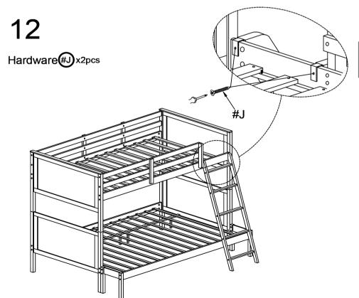
Use Screw (#J) to secure the ladder to the bed.
