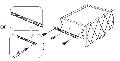
Loosen the guide screw and adjust to make the drawer level.
