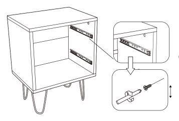
Loosen the guide screw and adjust to make the drawer level.
