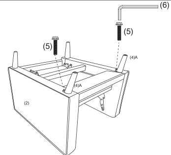
Attach 2 rear feet (Part 4A) to seat frame (Part 2) using Bolts (Part 5) x 2. Use Allen Wrench (Part 6) to tighten the bolts.
