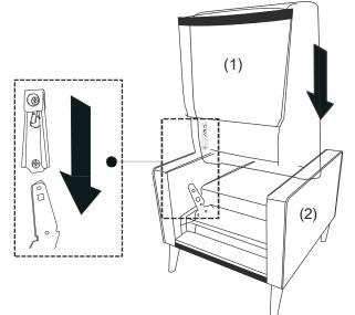
Slide the metal brackets on back cushion (Part 1) into the metal glides on seat frame (Part 2). Lower the back cushion onto the seat frame until it locks into place. Pull down the fabric flap and attach to the chair using the hook and loop system.
