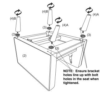
Using Plastic Washers (Part 3) x 4, attach Rear Feet (Part 4A) x 2 & front feet (Part 4B) x 2 by rotating clockwise to tighten.
