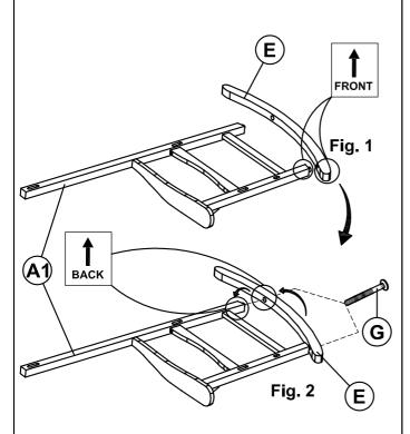
Attached each rocker (E) to right and left side frame (A1 & A2) as picture shown, connecting front of rocker to front legs first then the back of rockers. Secure connections with 1 3/4" Bolts (G).
