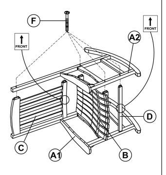
Install Seat (B), back support (C), and Apron (D) into corresponding holes of right side frame (A1). Attach the left side frame (A2) onto seat (B), back support (C), and apron (D). Secure left side frame (A2) using 1 1/4" bolts (F), as shown.
