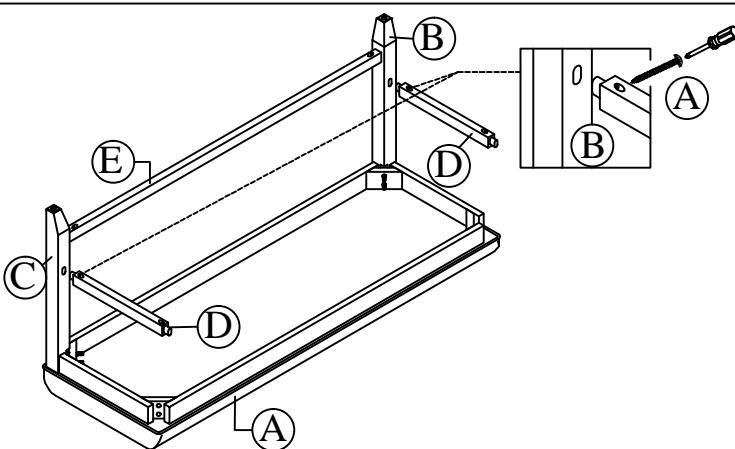
Step 2: Attach the Side Stretcher (D) to the Bench Leg (B);(C) by inserting Pan-Head Screw (4) and tighten with phillips-head screwdriver (not provided). Do not fully tighten.
