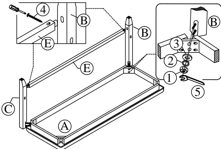
Step 1: Attach Left Bench Leg(B) and Right Bench Leg (C) to the corner block of the Seat Box w/ Seat Cushion (A) by inserting Hex Nut (1), Lock Washer (2), Flat Washer (3) and tighten with Wrench (5). Attach the Long Stretcher (E) in the middle of 2 Bench Leg (B);(C) by inserting Pan-Head Screw (4) and tighten with phillips-head screwdriver (not provided). Do not fully tighten.
