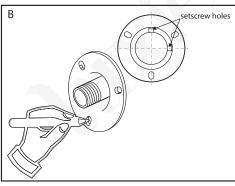
B. Place mounting base on the wall as shown in the figure with setscrew holes set at 12 and 3 o'clock positions. Mark the placement for the 3 screws with marker.
