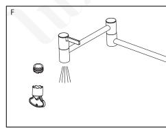
F. Remove aerator from the spout and turn on the water to flush out any debris in the plumbing system. Also check for leaks at all connections. Install the aerator when done. The installation is now complete.
