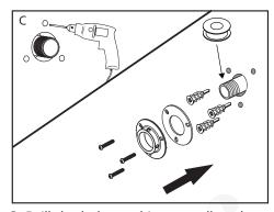
C. Drill the holes and insert wall anchors into the holes. Apply PTFE tape onto the nipple in counter-clockwise direction. Secure the mounting base with the supplied screws.
