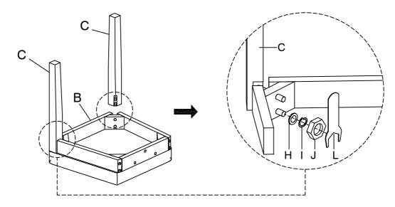
Take the spanner, and turn the washers to the corner blocks until the legs are secured. DO NOT TIGHTEN COMPLETELY. Stop when you feel you are adding force to tighten the washer.
