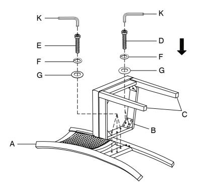
Stand the chair up on an even surface and check that it is balanced. If there is a slight wobble, apply downward pressure in the corner where a leg is uneven. Keeping pressure in that corner, tighten all bolts. If balanced, apply downward pressure evenly in the center and tighten all bolts. Do not over-tighten beyond hole depth.
