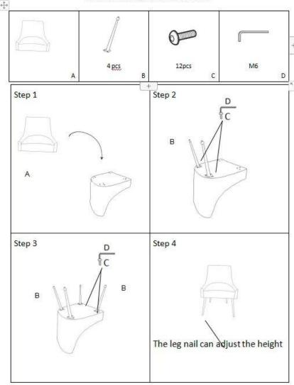
${f Note}$ : Put all the screws into the hole site, And then tighten them. Do not tighten one by one
