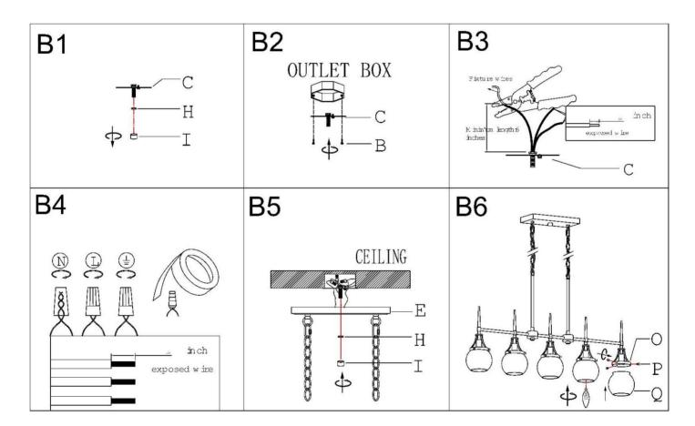
Step B1 » Unscrew hex nut (H) and cap nut (I) from single bar (C).
