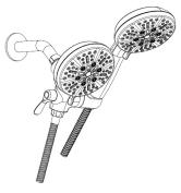
® Place hand-held shower head in rotatable holder. Point all shower heads away from you and turn on the water full force. Check for leaks. Re-tighten all connectors if necessary.
