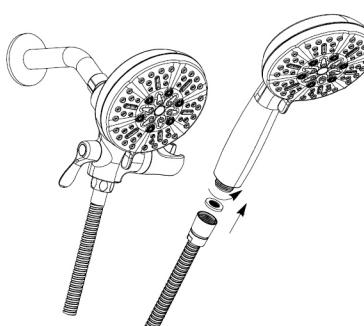
⑦ Locate the hose end with short hose nut and hand tighten to shower head. **IMPORTANT!** If hose is not installed in this manner unit will not operate properly.
