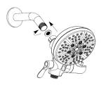
6 Attach 3 in 1 fixed mount shower head by threading clockwise onto shower arm with rotatable holder to the right and 3-way diverter control handle to the left. Use a wrench to tighten shower head nut to a snug fit. Do not over tighten. Wrap shower head nut with a cloth if you are using pliers.
