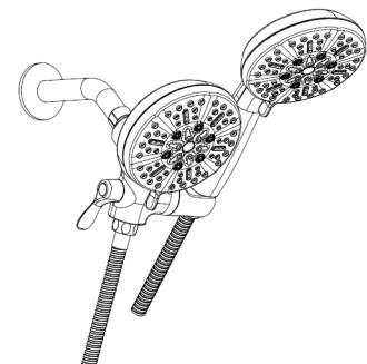
⑧ Place hand-held shower head in rotatable holder. Point all shower heads away from you and turn on the water full force. Check for leaks. Re-tighten all connectors if necessary.
