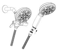
② Locate the hose end with short hose nut and hand tighten to shower head. IMPORTANT! If hose is not installed in this manner unit will not operate properly.
