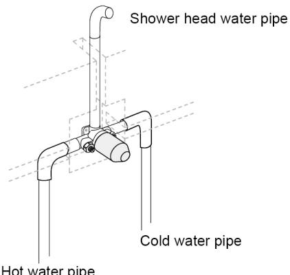
③ Connect water pipes to shower valve body as picture shows. And then install the shower valve body with screws.
