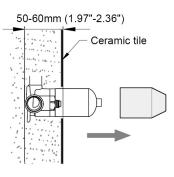
④ Switch on/off the cartridge, check all connectors without any leakage. And then seal the wall and take off protection cover.
