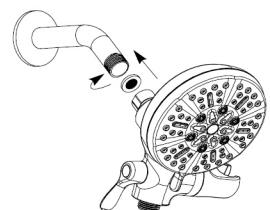
⑥ Attach 3 in 1 fixed mount shower head by threading clockwise onto shower arm with rotatable holder to the right and 3-way diverter control handle to the left. Use a wrench to tighten shower head nut to a snug fit. Do not over tighten. Wrap shower head nut with a cloth if you are using pliers.
