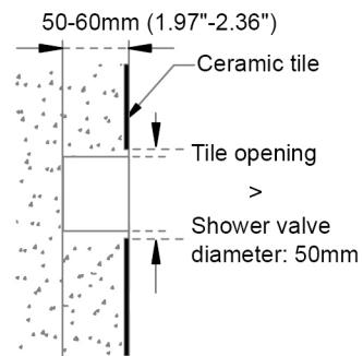
① Use special tools to chisel holes on wall for installing, shower valve body and water pipe.
