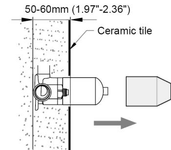
④ Switch on/off the cartridge, check all connectors without any leakage. And then seal the wall and take off protection cover.
