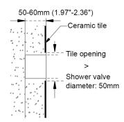
② Recommended depth for installing shower valve body before tiling tiles: 50-60mm (1.97"-2.36"). Note: Tile opening should be bigger than shower valve diameter at least 5 mm.
