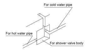
① Use special tools to chisel holes on wall for installing, shower valve body and water pipe.
