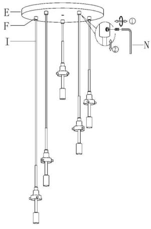
5 » If needed, shorten the extra length of the fixture wires from cord (I) so that they all are at least 6 inches (152.4 mm) long above canopy (E) within the outlet box.
