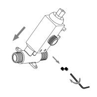
3.Put the plastic protected cover on the thread side of 3 ways body; Connect water pipes to 3 ways body as picture shows, then fix the 3 ways body with screws.
