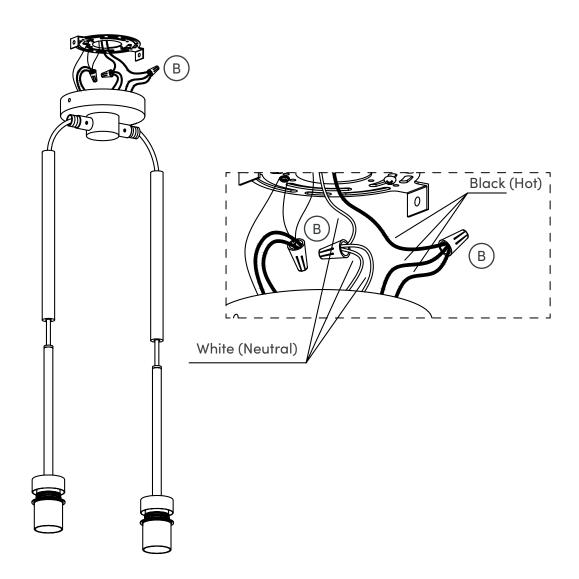
Secure the Fixture (2) to the Mounting Plate (C) on your pre-installed electrical box using the M4\*15mm Screws (D).
