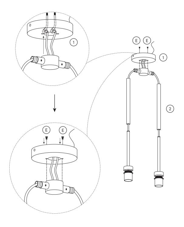
Allow cords to hang or rest freely, then secure the set screws to hold the cords at your desired length.
