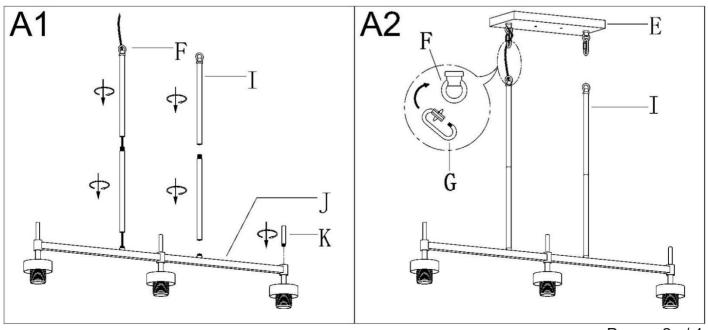
Step A1 » 1) Carefully pass the fixture wires through one side of loop (F) and tubes (I).
