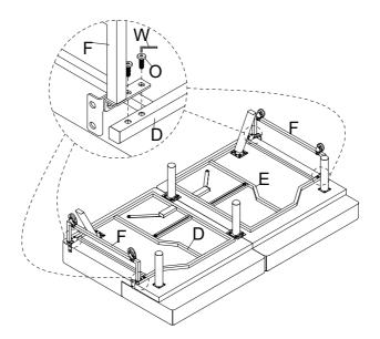
Push the back of Sofa (A) to the highest position. Then move Left & Right Bottom Frame (D & E) and Wheel Frame (F) to the front as shown.
