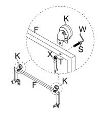
Attach the Wheel Frame (F) to the Left & Right Bottom Frame (D & E), insert the Bolt (O), turn the L-Allen Key (W) to tighten them.
