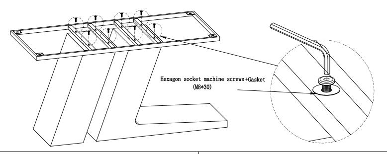
2. Place the desktop on the top of the support frame and align the ears of the support frame with the holes of the bottom plate of the desktop, put in the hexagonal machine wire and gasket and tighten it with a wrench
