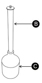
Screw metal leg B to the top of wood base C as shown above.
