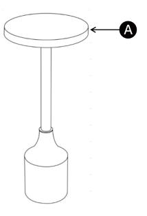
Screw metal leg B to the bottom of table top A as shown above.
