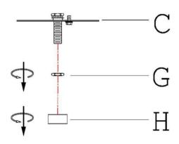
4 » Secure single bar (C) to the outlet box with mounting screws (B).
