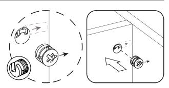
Using a screwdriver, you will turn the cam lock until it stops, usually between 130° or 180°. You will feel the panels pulling closer until they are secured.
