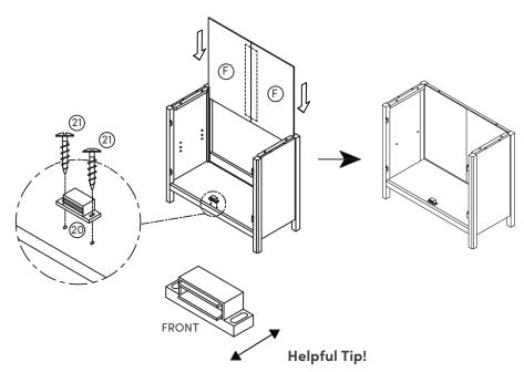
Magnetic Door Catch can be adjusted front to back to solve for proper door alignment.
