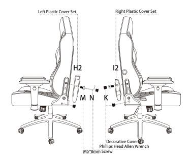
Attach the Left Plastic Trim Cover (Part H2) and Right Plastic Trim Cover (Part I2) using (2) M5\*8mm Screws (Part M). Tighten using Phillips Head Allen Wrench (Part N). Insert(4) Decorative Covers (Part K).
