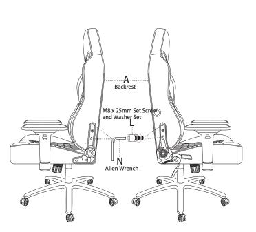
Attach the Backrest (Part A) to the Seat using (4) Set Screw and Washer Sets (Part L) These are preinstalled in the back. Tighten with Allen Wrench (Part N).
