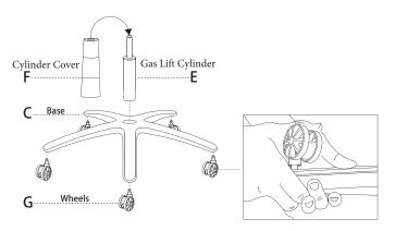
Insert (5) Wheels (Part G) into the Base (Part C). Insert the Gas Lift Cylinder (Part E) into the Base. Slide the Cylinder Cover (Part F) over the Gasl Lift Cylinder.
