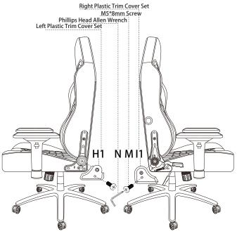
Attach the Left Plastic Trim Cover (Part H1) and Right Plastic Trim Cover (Part I1) using (2) M5\*8mm Screws (Part M). Tighten using Phillips Head Allen Wrench (Part N)
