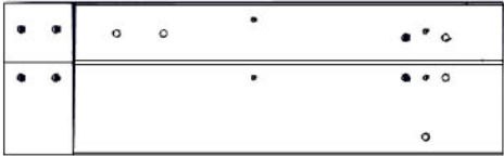
J03 JOIST ASSEMBLY - W2A03550 (x1) 1 7/16"x8 7/16"x28 7/16" (36x214x722)
