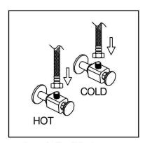
5. Attach flexible hose to water supply.
