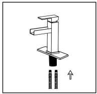
2. Screw and hand tighten the hot and cold flexible hoses to the faucet. DO not use a wrench to tighten hoses as this may damage the hose and/or the hose threads.
