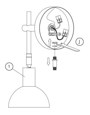
Place the plastic plug inside the hole in the bottom of the fixture that the small stem filled originally.
