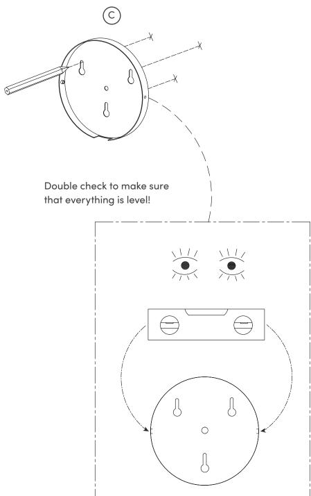
Using a 1/4" (or 6mm) Drill Bit, drill your holes for the wall anchors to be placed in.
