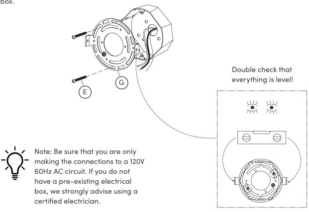
Wrap the ground wire from the Fixture around the grounding screw on the Mounting Plate (G) & then secured by tightening the screw.
