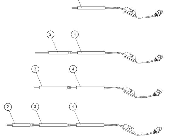
Thread the cord back into the Fixture (1).
