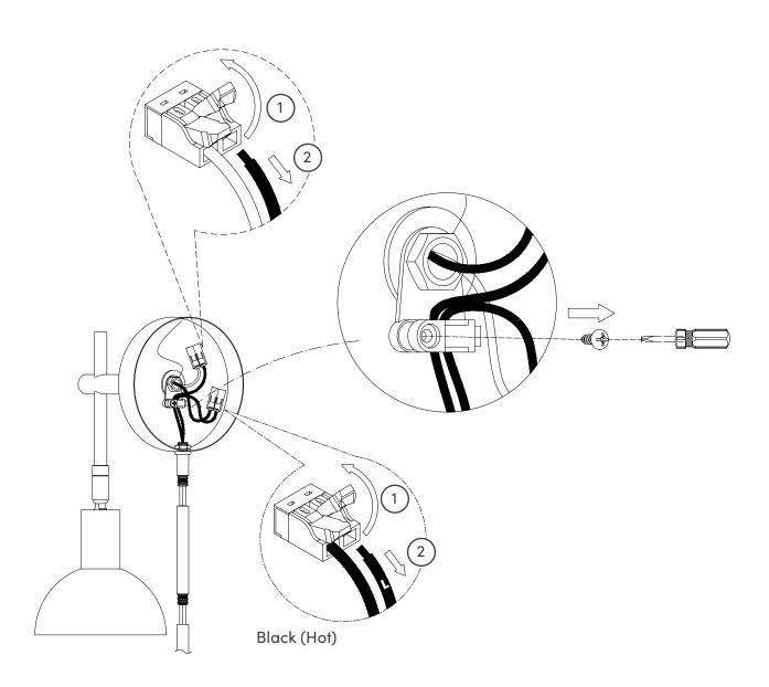
Remove the cord with the plug from the bottom of the fixture.
