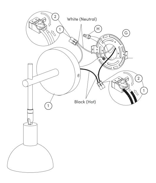
Last step! First secure the Fixture (1) to the Mounting Plate (G). Once fully secure, then install a light bulb (not included) and voila!
