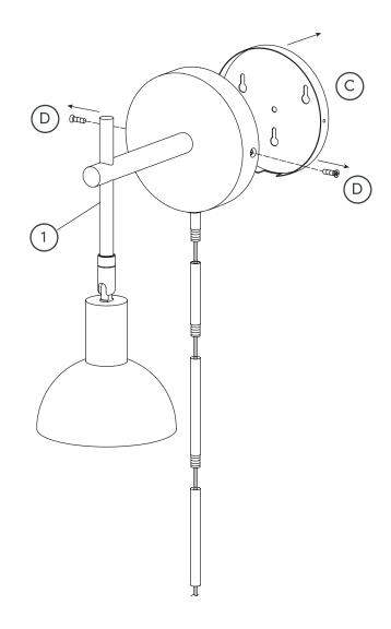
Remove wires that run to the plug from each wire connector component in order to allow the cord to be released out the bottom of the fixture.
