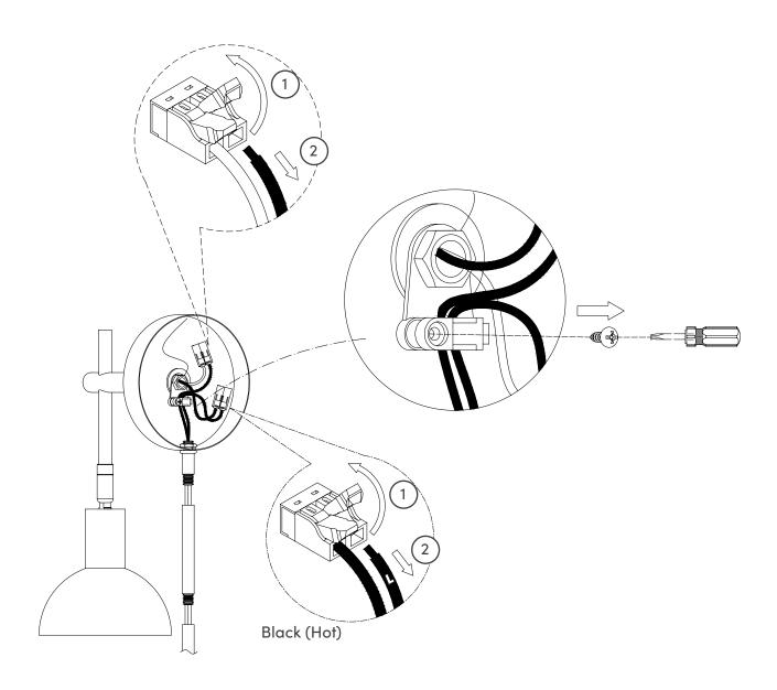
Remove the cord out the bottom of the fixture in order to install the decorative cord stem at its desired length.
