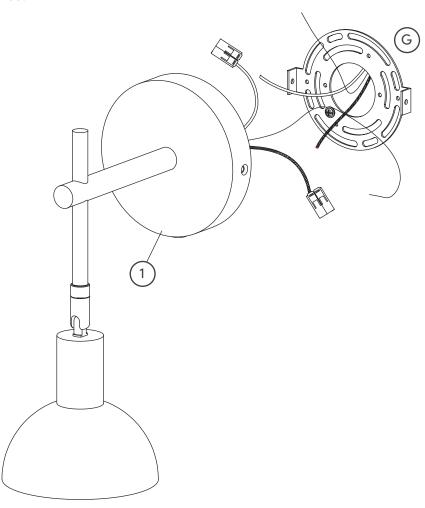
Okay, let's get back to it! Use wire connectors to connect the matching colored wires (White to White, Black to Black). Use the Wire Nuts (H) to connect the ground wire from the Electrical Box to the Ground wire from the Fixture (1).
