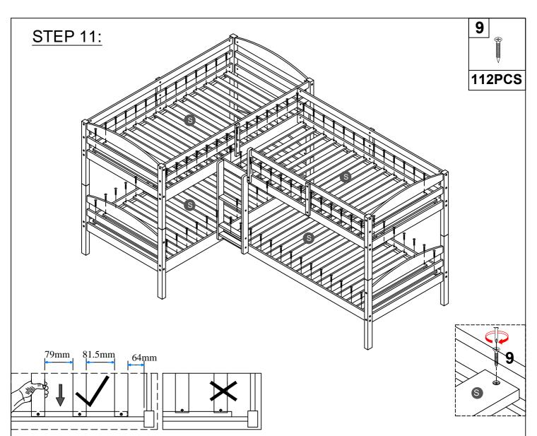
Note: Do not lock the screws of the bed slats to the outermost edge of the bed slats, you need to leave a certain space at the edges, otherwise it will cause the board to break. Do not lock the bed slats on the edge of the wood, please hold firmly before screwing, hold it in place with one hand, then lock the screw.
