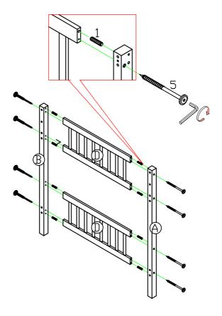
No TE: In this step, DO NOT tighten any bolt until you connect all part together
