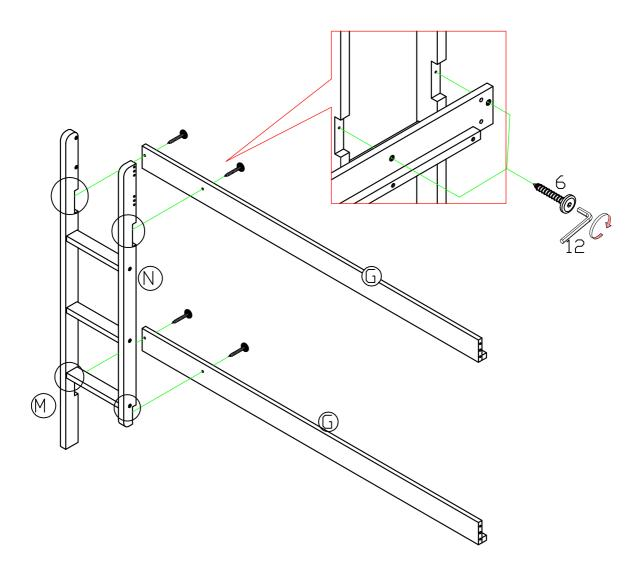
No TE: In this step, DO NOT tighten any bolt until you connect all part together
