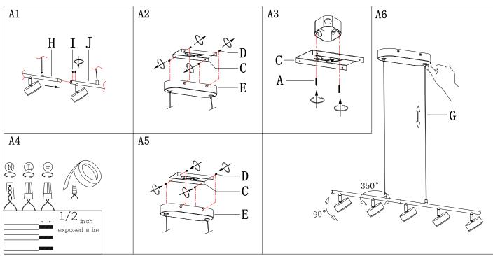
Step A1 » Insert fixture body-A (H) into fixture body-B (J), then secure them with small screws (I).
