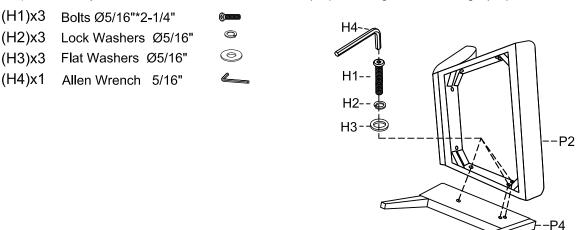
Step 3. Loosely attach the assembled seat cushion (P2) to the left arm with legs (P3) as shown.
