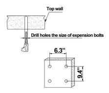
4). Insert the shower fixed seat into the four expansion bolts to adjust the nuts to fit the ceiling is on the same plane, and finally Finally, the square hole ceiling is buckling up to the suspended ceiling board.
