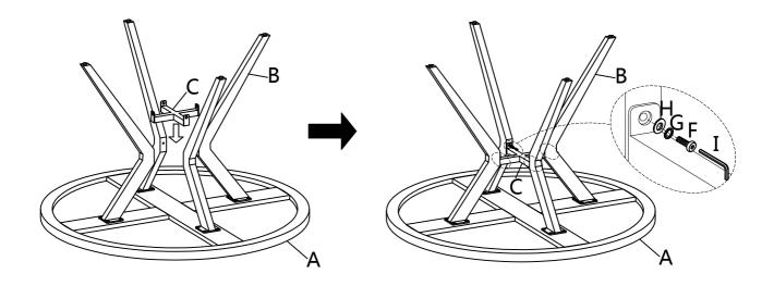
With assistance from your adult partners, turn the Dining Table right way up. Adjust the pre-installed levelers on the bottom of Leg (B) until the Dining Table is level with the ground.
