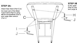
STEP 5B: Attach Seat Back (Part C) to the upper part of the Metal Tube Frame (Part A) using M6\*35 Screws (Part H) and Large Allen Wrench (Part J)
