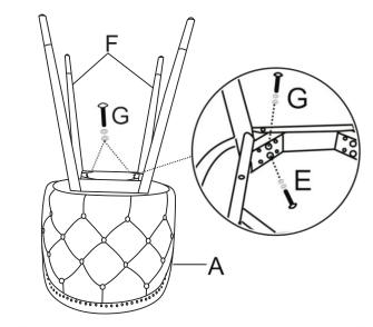
Put the screws in the holes, tight the screws,but not too tight,90% is ok.
