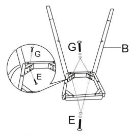
Put the screws in the holes, tight the screws, but not too tight, 90% is ok.
