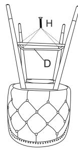
Put the screws in the holes, tight the screws,but not too tight,90% is ok.
