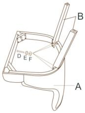
Put the screws in the holes, tight the screws, but not too tight,90% is ok.
