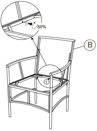
Secure a spring washer (2) and a bolt (1).
