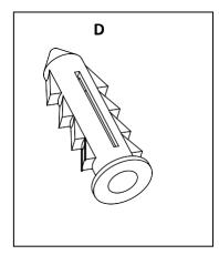
(Anchorsize-13 mm head dia x 40 mm length)
