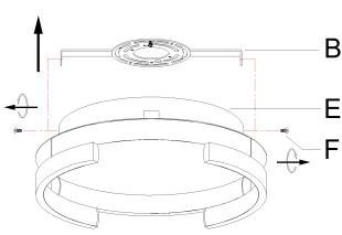
4 » Attach mounting plate (B) to the outlet box with mounting screws (D).
