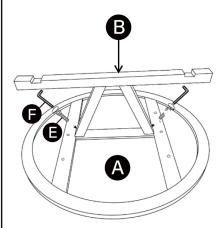
Flip the table top upside down, attach wood base B to the table top A using bolts and flat washers.
