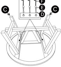
Attach wood base C to the table top A using bolts and flat washers.
