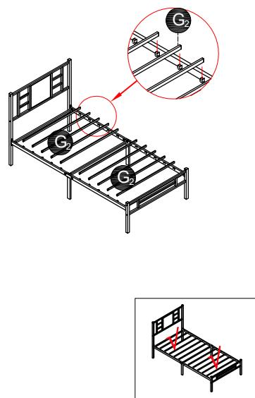
7 Check and tighten all screws
