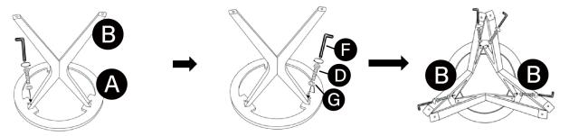
Don't fully tighten the screw, leave screw loose for adjustment (only 1-2 turns to hold the leg in place).
