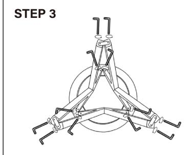
After all components are assembled, go back and fully tighten all the screws to ensure all components are firmly attached.
