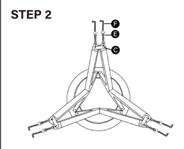
Fasten the other end of the legs B together with SHORT-ER screws E and flat connector plates C.
