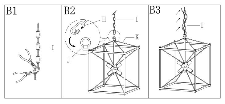
Step B1 » By measuring, determine the correct number of links needed for proper hanging height. Using the chain pliers, disconnect and discard the unwanted part.
