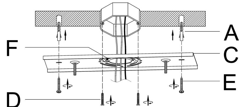
**Step 4:** Fix the Anchor Screw(A) to the ceiling and the Mounting Bracket (C) to the junction box through Mounting Screws (D) and Tapping Screws (E)
