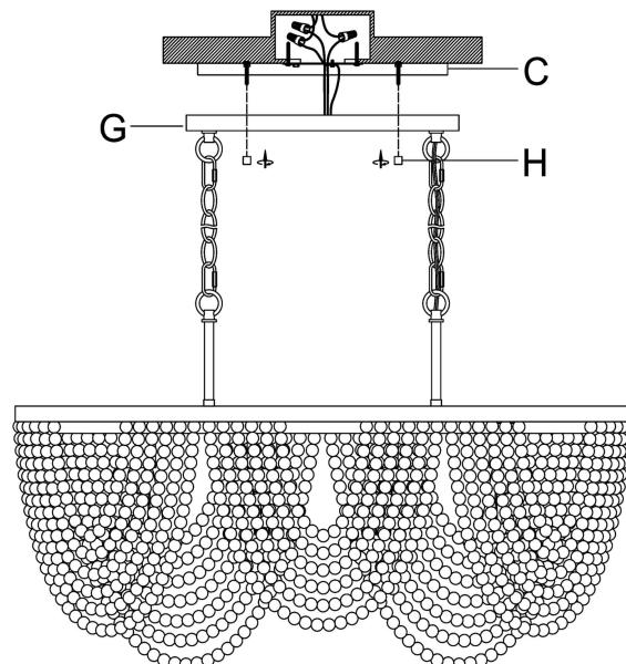
**Step 5:** Attach the Canopy(G) to the junction box and fix it by turning the Canopy Nut(H) clockwise.
