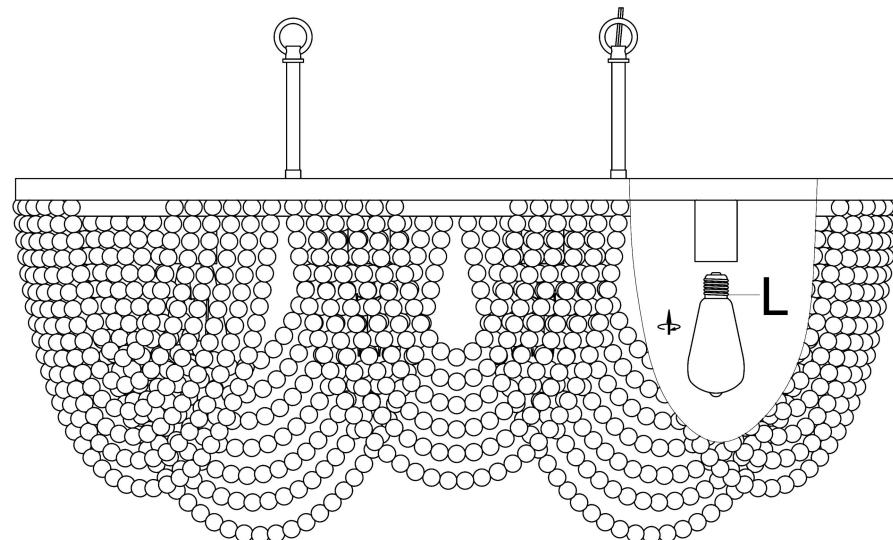
**Step 6:** Insert the bulbs (L) into the Sockets
