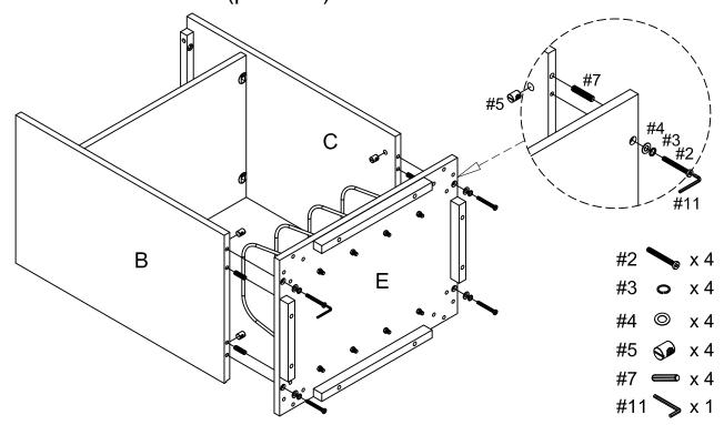
Step 5. Attach legs (part G) to bottom panel (part E) using wood dowels (part #7), short bolts (part #1), spring washers (part #3), flat washers (part #4) and allen wrench (part #11).
