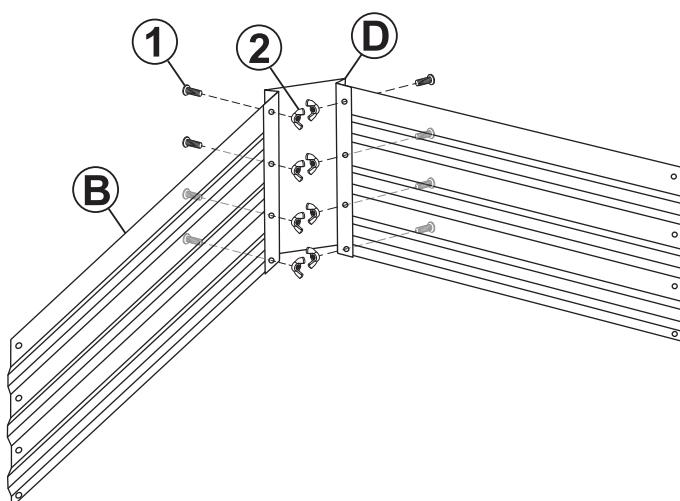
Align two Medium Panels (B) with one Corner (D) and secure using eight bolts and wing nuts.
