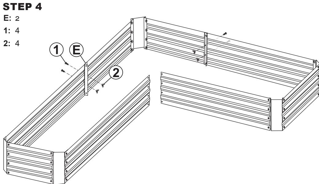
**IMPORTANT:** Do not install hardware into the top and bottom mounting holes.
