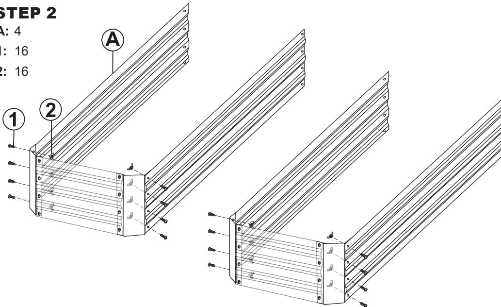
Ensuring the rolled edges are facing the inside of the garden bed, align Long Panels (A) with the end panel corners and secure using four bolts and wing nuts.
