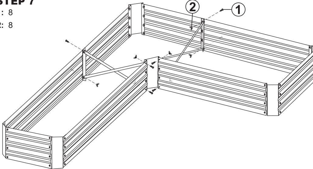
Secure the top and bottom of each bracket with bolts and wing nuts.
