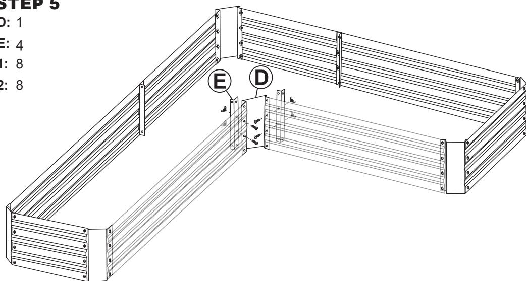
Ensuring the corner piece is facing inward, align one Corner Panel (D) and two Brackets (E) with the long panels.
