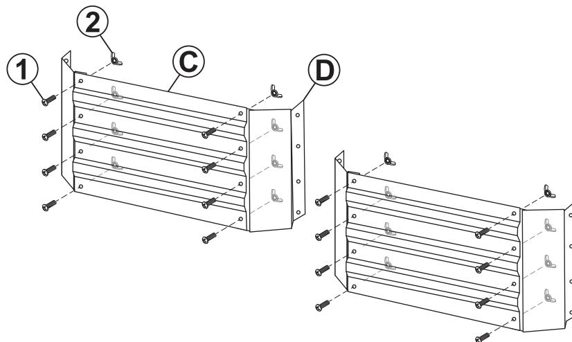
**IMPORTANT:** Identify the rolled edges of the panels and ensure they are installed facing the inside of the garden bed.
