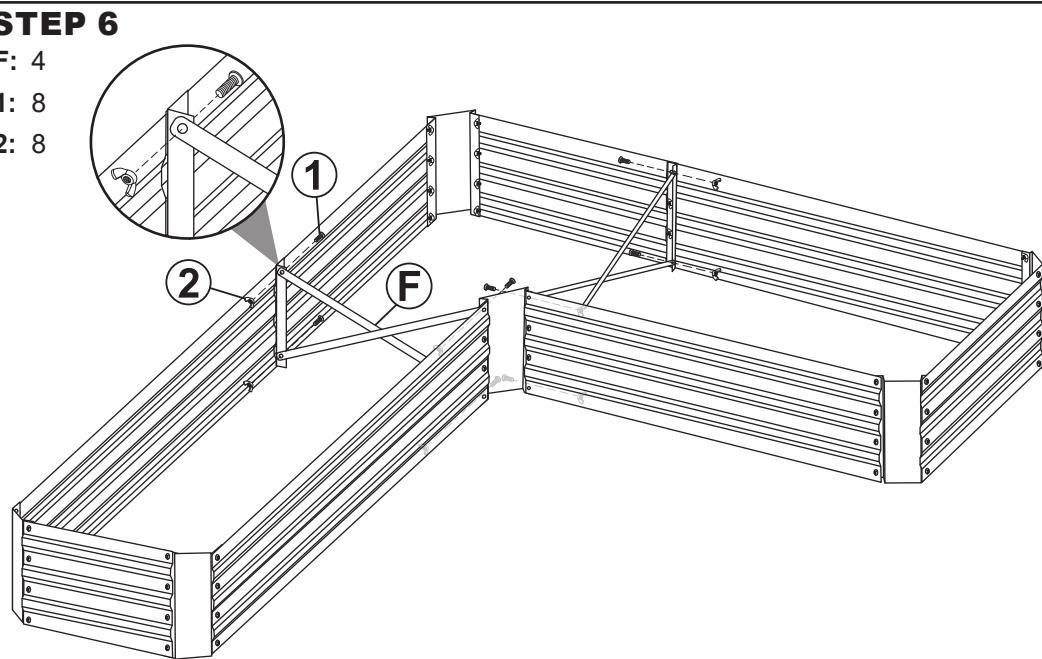
**IMPORTANT:** Ensure the bolt is installed in the correct direction, with the wingnut on the outside of the bracket as shown.
