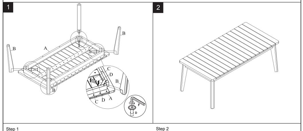
Attach Leg (B) to Table Top (A). Use Bolt (C) and Washer (D) tighten with Allen Key (F).
