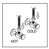
5. Attach flexible hose to water supply.
