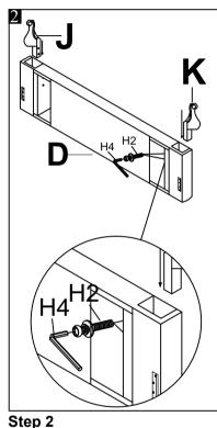
Attach wood legs "J" & "K" with footboard "D". Using wrench (H4) to lock with bolts "H2".
