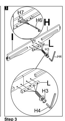
Attach wood bar "K" to the 2 rails "H" & "I".Using Allen key (H4) to lock with bolts "H3". Lock the both side rails ( H & I) (front & rear of rail) tight and alignment with metal plate (H7) by using 8x screws (H6)
