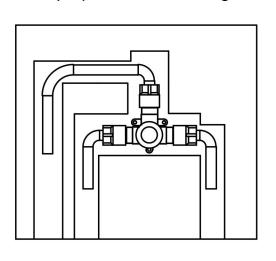
4. The wall is slotted and then drilled.
