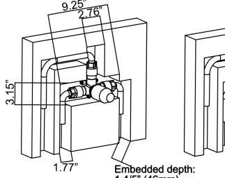
5. Drive the rubber plug into the wall, and fix the main body to the wall with screws.
