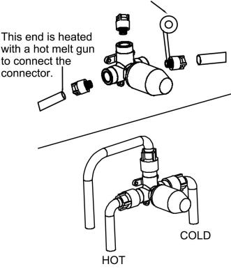
3. Put the valve body connected with the pipe against the wall, draw the outline with a pen and prepare for the slotting.
