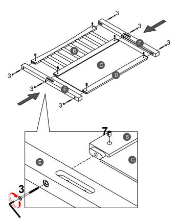
Note:Part 7 will face up with the "x" mark on it, otherwise it cannot be tightened
