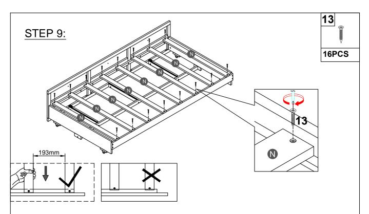
Note: Do not lock the screws of the bed slats to the outermost edge of the bed slats, you need to leave a certain space at the edges, otherwise it will cause the board to break. Do not lock the bed slats on the edge of the wood, please hold firmly before screwing, hold it in place with one hand, then lock the screw.
